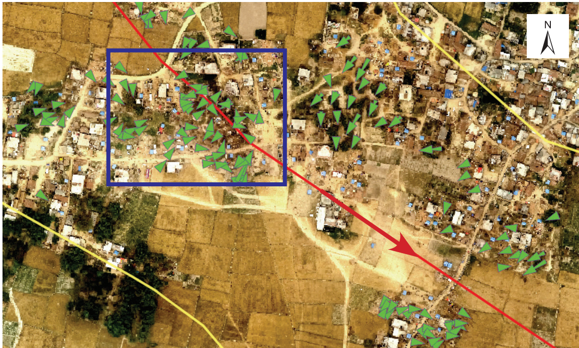
Figure 3.7a: Wind pattern associated with tree fall at Purainiya, Pheta. Note: Green arrows indicate direction of the wind but not the magnitude. Red line: center and direction of tornado path.
