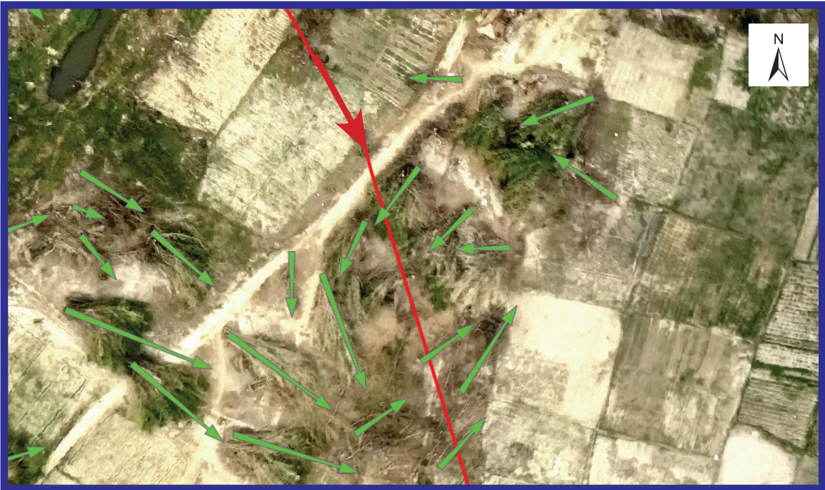
Figure 3.6c: Zoomed view of the region in blue box in Figure 3.6b, indicating anticlockwise circular wind pattern associated with tree fall. Green arrows indicate direction of the wind but not the magnitude. Red line: center and direction of tornado path.
